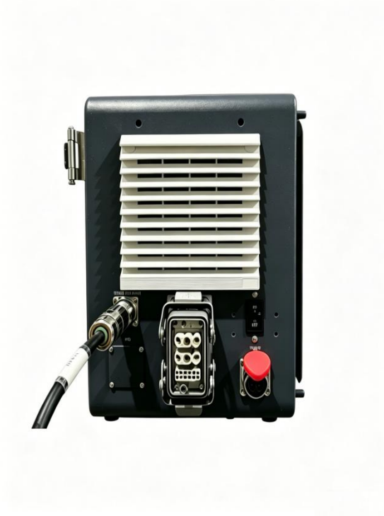
Figure 5-5 Connection of Handheld Unit or Teach Pendant to Controller
