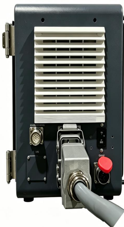
Figure 5-4 Connection of Robot Body Cable to Controller
