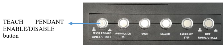
Figure 5-6 Position of TEACH PENDANT ENABLE/DISABLE button
